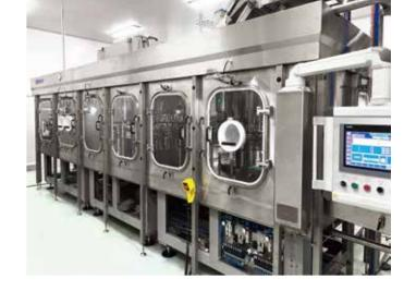
The Blowing-Filling-Capping Combiblock is one powerful combination, which completes the whole process from preform to bottled, It can decrease intermediate links such as conveying, empty bottle handling, stacking and storage processes, improve packaging sanitary conditions, reduce cross-contamination, increase overall operating efficiency, save energy consumption, so that it cuts overall production costs
