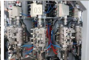
The maximum 1-cavity capacity of the bottle blowing machine can reach 2500BPH/Water Bottles, 2000BPH/CSD Bottles,
